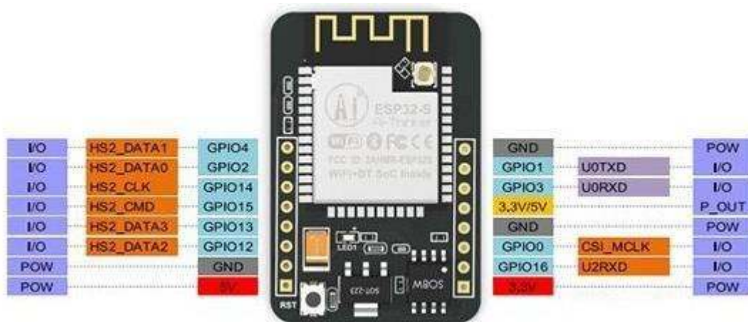
Figure 3.1: Pin configuration of an ESP 32 Camera
