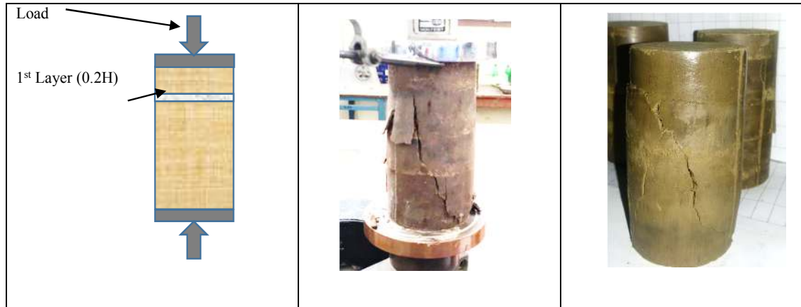
Figure 4. Reinforced clayey soil sample for UCS test with 1 st layer of geosynthetics at 0.2H
