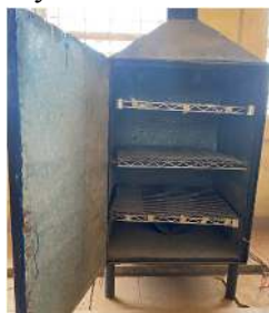
Plate 3: Cabinet dryer: Developed by Olawuni Moses FUTA.
